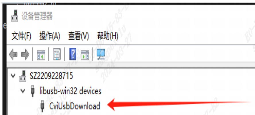
Fig. 3.2: Verify if the driver installation is correct
