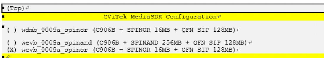
Finally, exit the selection and save the settings (they will be stored in. /build/.config) to complete the selection of the SDK compilation configuration.
