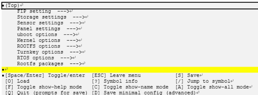
The configuration process can be set/returned by [Enter] [Space] [ESC]
