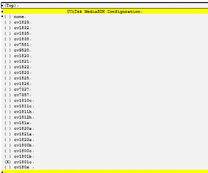
The EVB version number will list the corresponding choices, and the selection of EVB will also specify the compiled image's DDR and Flash size (for this example, the selected EVB comes with DDR3 and 16MB of SPINOR Flash).
